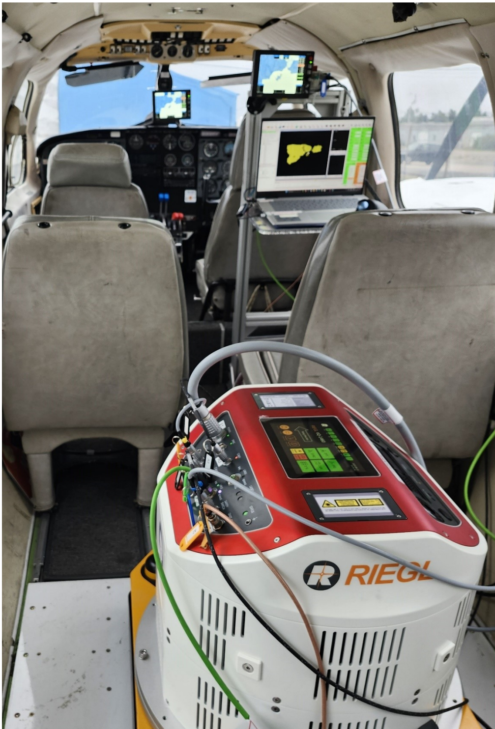
Figure 1: IGI CCNS-5 with RIEGL VQ-1460 in Piper Cheyenne from XEOS Imagerie
