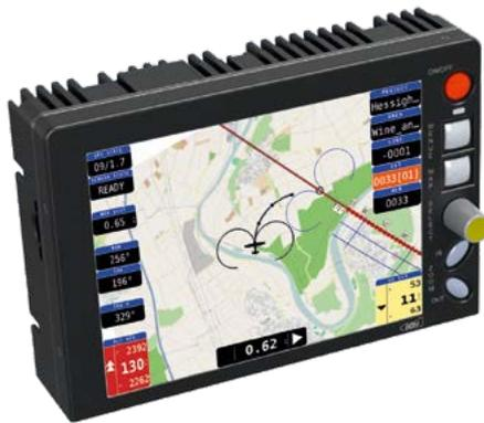
The **Computer Controlled Navigation System - CCNS** - today is one of the leading solutions for aircraft guidance and sensor management.
