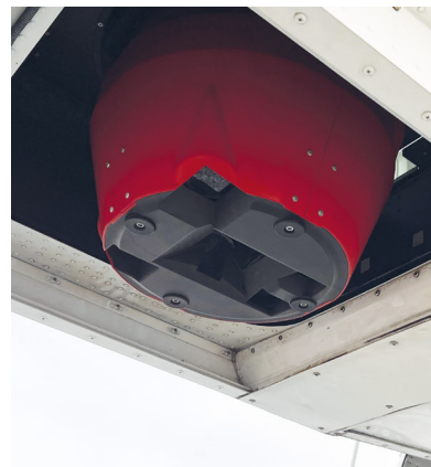
IGI URBANMAPPER-2 Performance installed in Cessna Caravan
