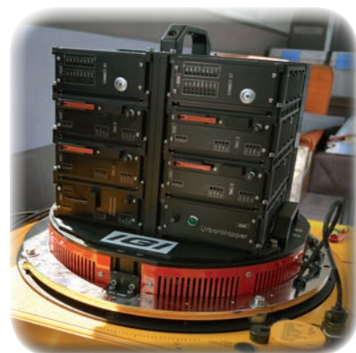
IGI UrbanMapper installed in stabilized mount GSM-3000
