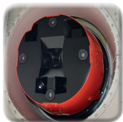
IGI UrbanMapper installed in fixed wing aircraft
