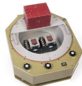
Example of Wild/Leica mount with mount adapter, IMU and two digital cameras..
